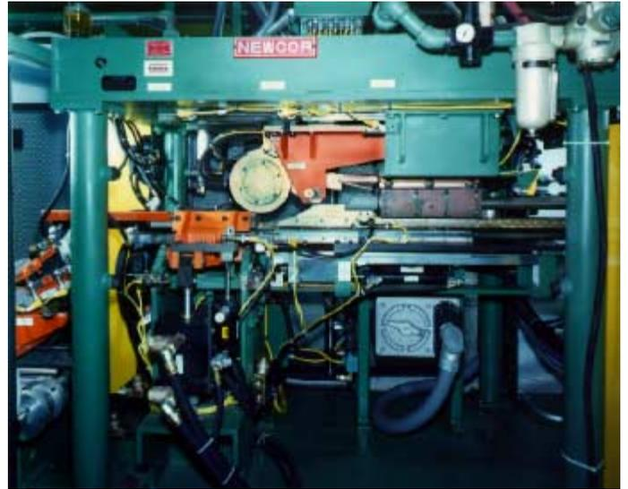
*This motor shell welder produces shells at a rate of 600 per hour.*
